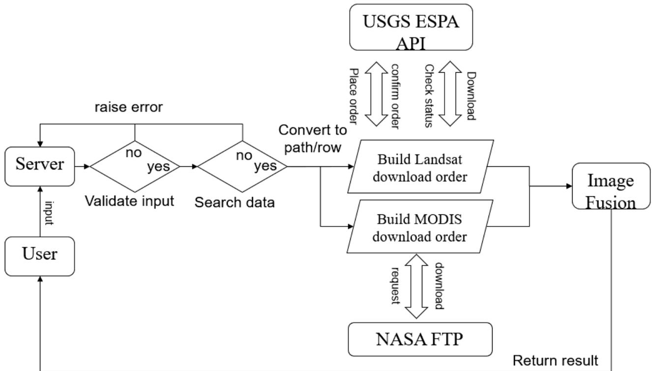
Fig. 2. Geoprocessing architecture for NRT MODIS image fusion
